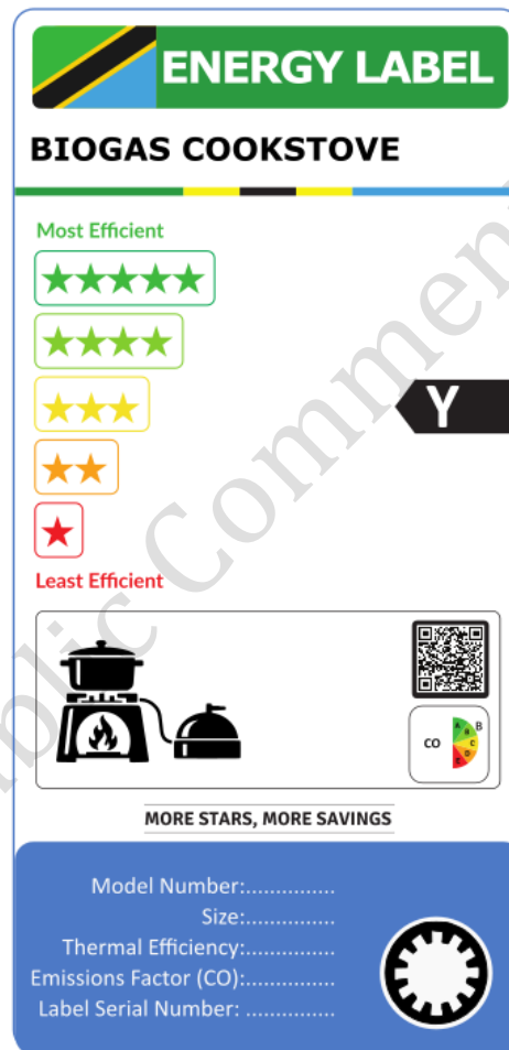
Figure A.1 Typical example for institutional BIOGAS CookStoves energy label
